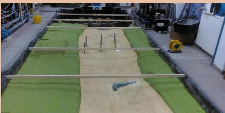
Fig. 2. Physical model with the bridges and elements of the river regulation
