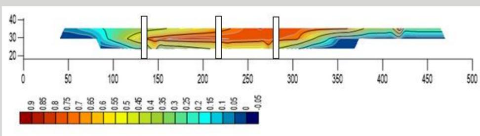
Fig. 5. Magnitudes of the flow velocities in bridge cross section
