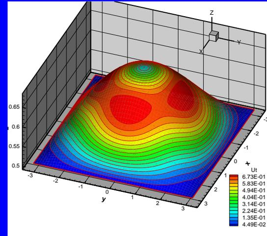
The 3D view of the surface shape and velocity magnitude distribution on the surface
