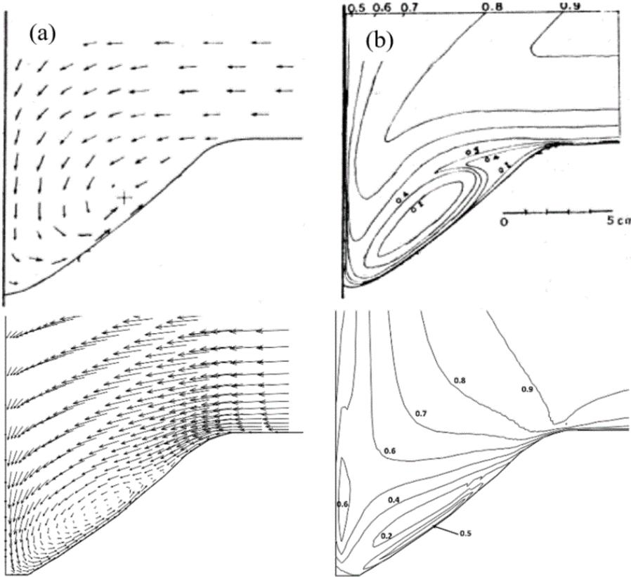
Comparisons of simulated and measure flow velocity in the vertical front plan of the scour hole
