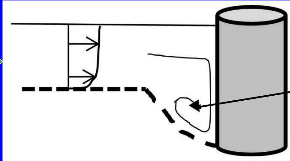
Additional Turbulence kinetic energy generated
