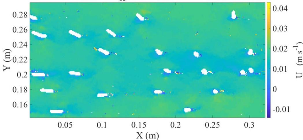
Test 2  $U_{\infty} = 0.02 \text{ m s}^{-1}$  - Longitudinal Velocity
