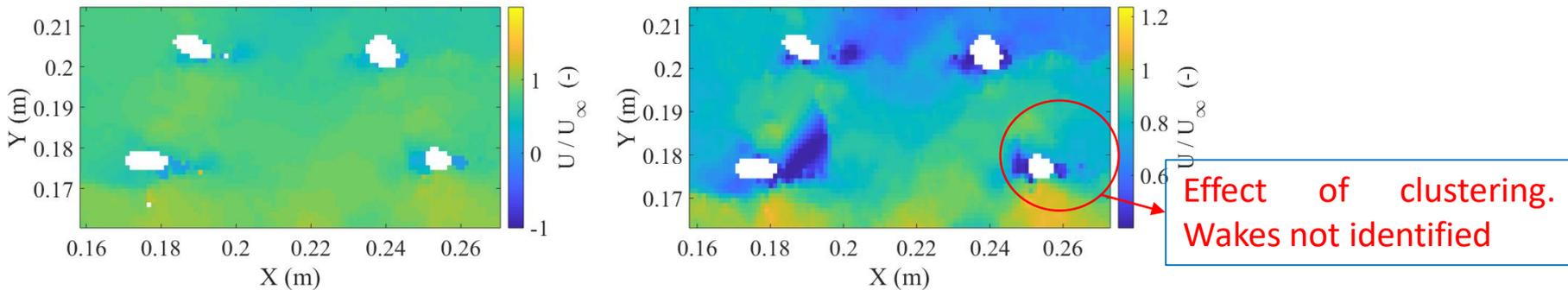
SP: Plots obtained from the tests with smaller particles produce plots with better quality and less outliers.
