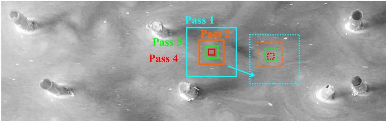
Resolution Analysis: Fine Resolution for the smallest possible velocity fluctuations, Intermediate Resolution for a conventional PIV window size, and a Coarse Resolution, which is equivalent to the ones used for SPIV.
