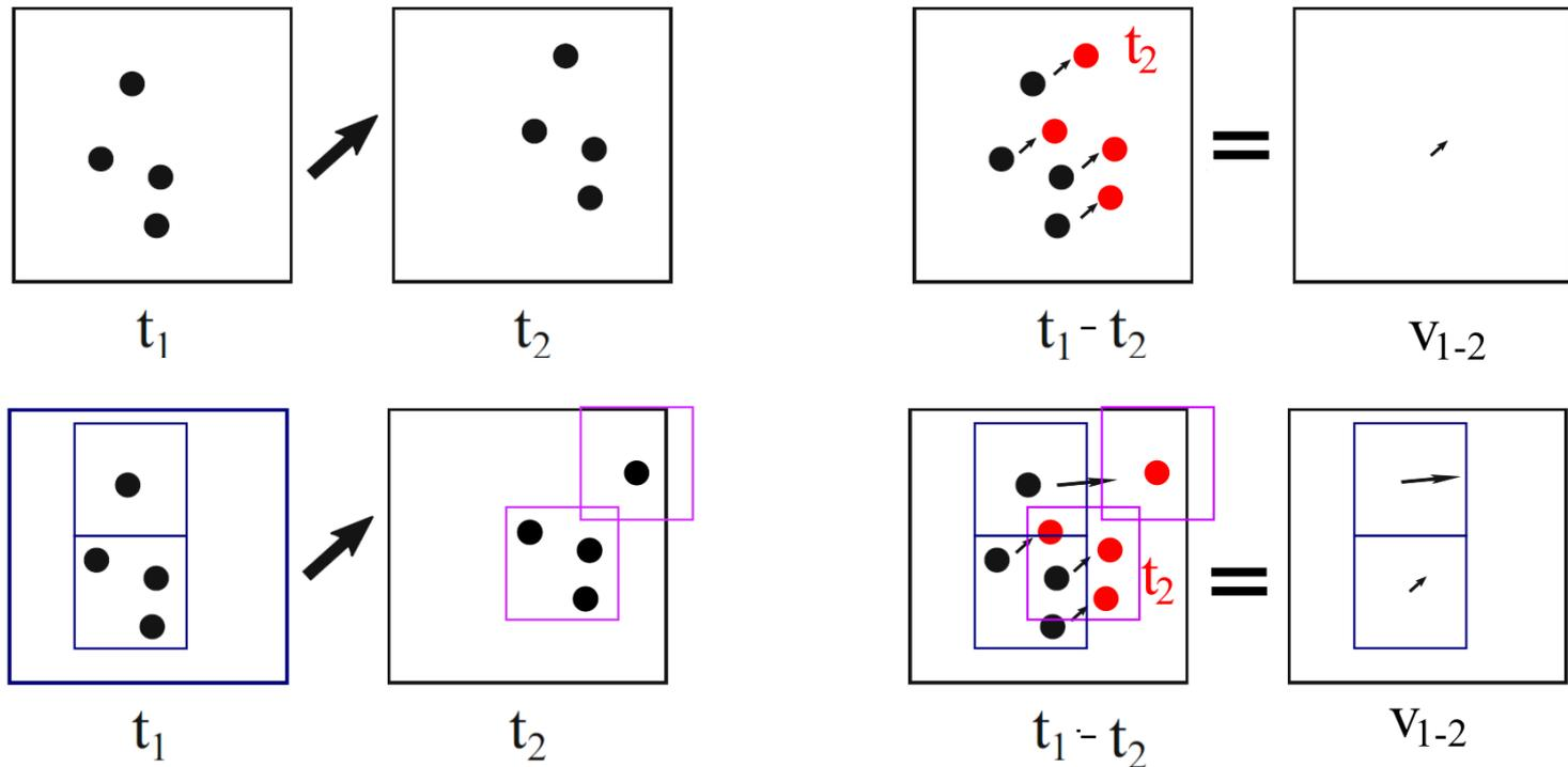
To capture a wider spectrum of velocities, correlations are computed sequentially with interrogation windows of different sizes. Each correlation with a single window size is called a pass.
