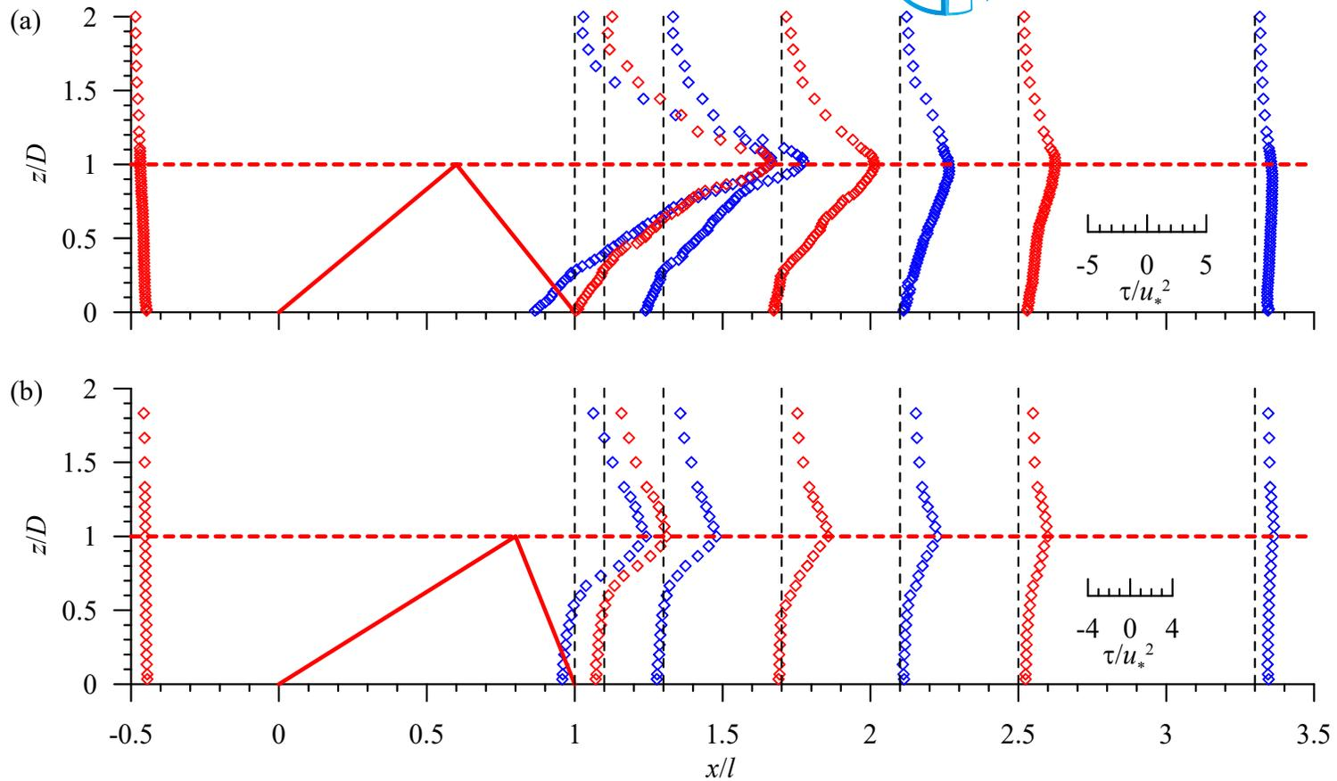
$\tau$  is the Reynolds shear stress relative to mass density  $\rho$  of water, defined by  $-\overline{u'w'}$
