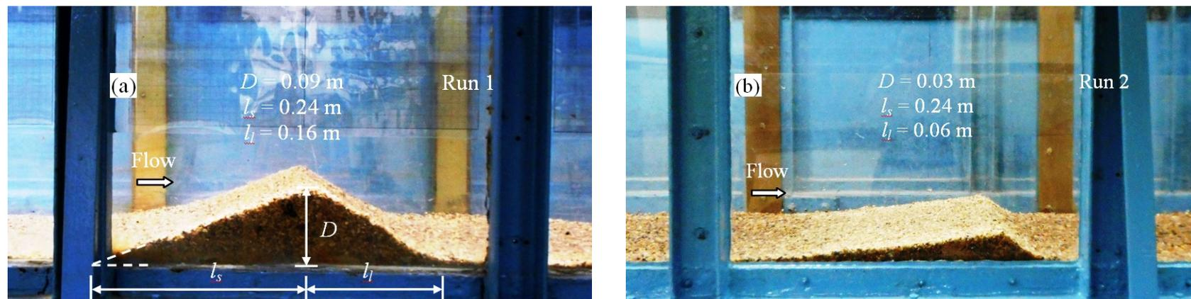
**Fig. 1** Photographs of the dunal structures for (a) Run 1 and (b) Run 2.
