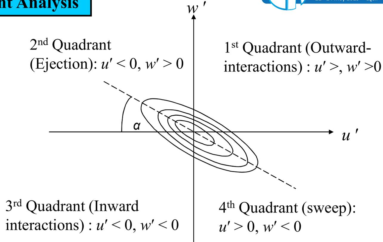
**Fig. 7** Quadrant plots of velocity fluctuations ( $u'$ ,  $w'$ ) on  $u'w'$ -plane.
