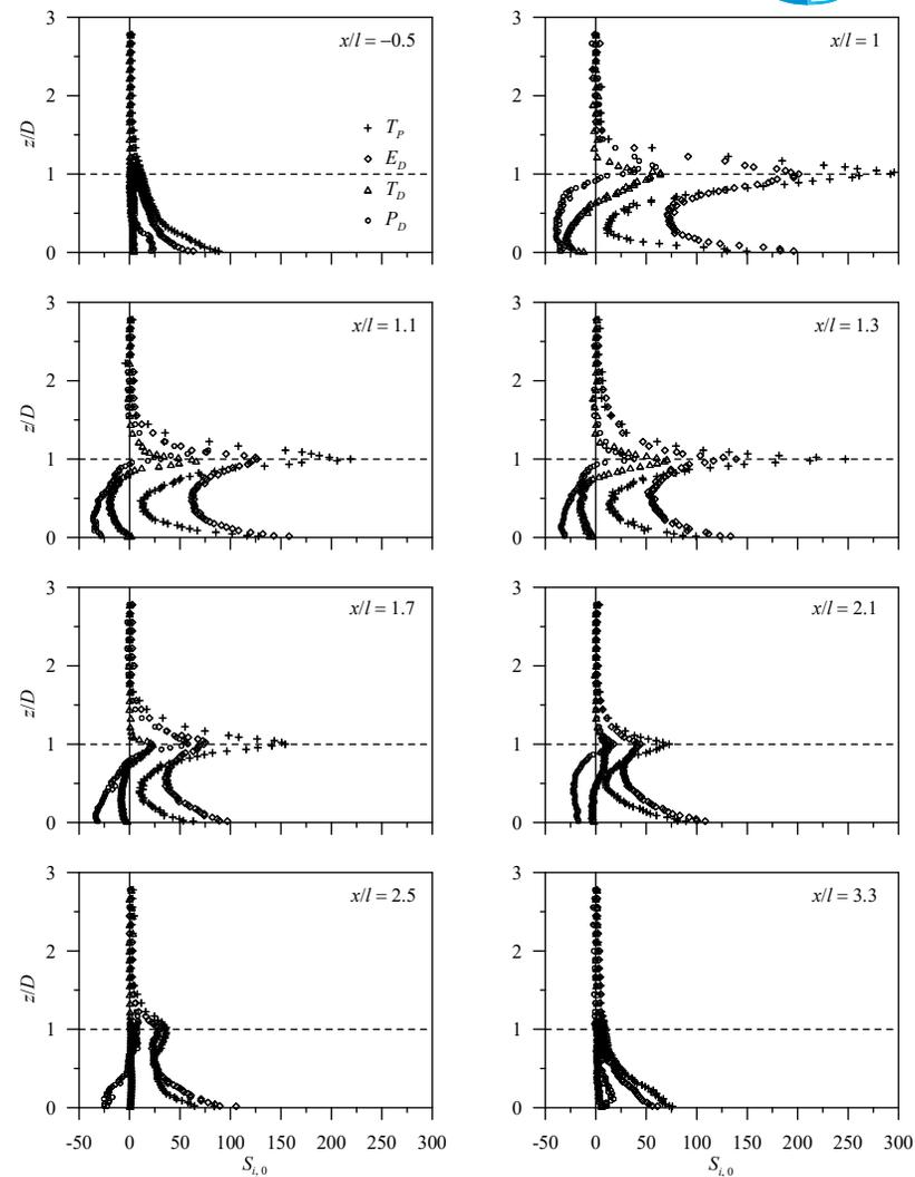
**Fig. 9** TKE budget components  $T_P$ ,  $E_D$ ,  $T_D$  and  $P_D$ , as a function of  $z/D$  at different streamwise distances for Run 1.
