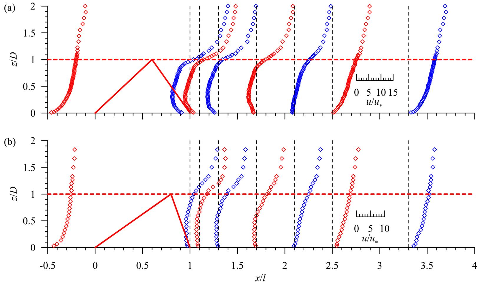
**Fig. 3** Vertical profiles of nondimensional streamwise velocity  $u/u_*$  at different streamwise distances for Runs 1 and 2
