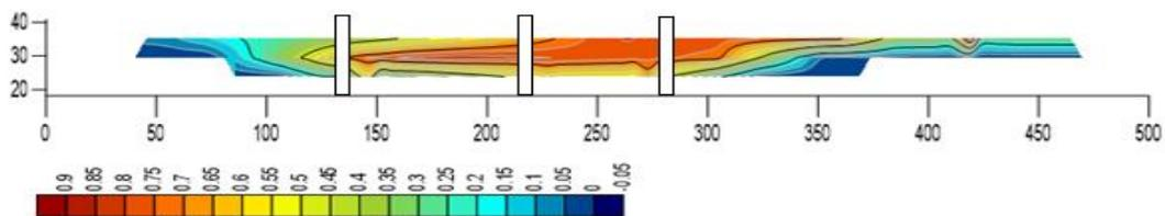
**Fig. 3.** Magnitudes of the flow velocities in bridge cross section
