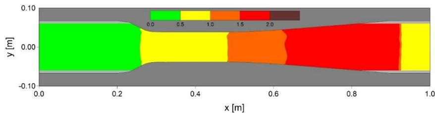
**Fig. 3.** Froude number [-] horizontal distribution (dimensions in meters).
