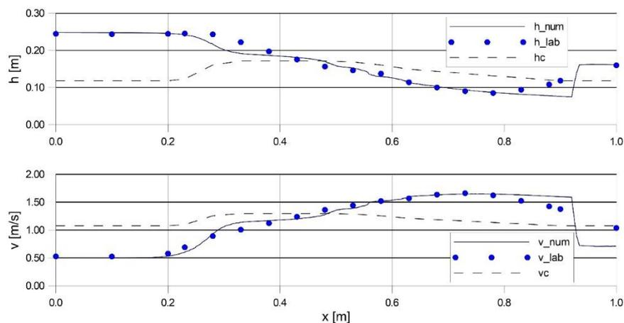
**Fig. 1.** Measured (lab) and calculated (num) profiles of water depth ( $h$ ) with the critical depth line ( $h_c$ ) and velocity ( $v$ ) with the critical velocity line ( $v_c$ ) along the channel constriction longitudinal axis.
