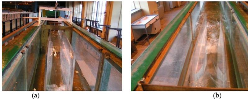
**Fig. 2.** Laboratory experiment in the channel constriction – downstream (a) and upstream (b) view of the transcritical flow.
