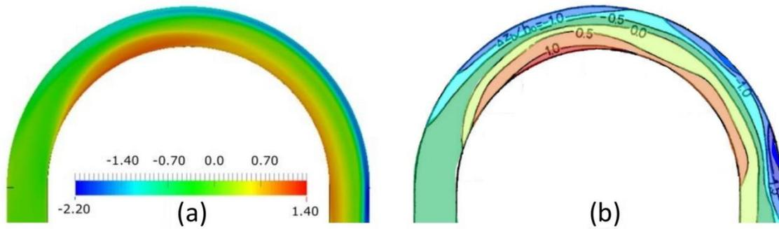
**Fig. 1.** Plan view of the normalized bed deformation; (a) simulation results using Wu's formula, (b) experimental data from the physical model.
