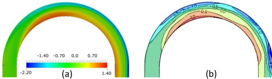
**Fig. 1.** Plan view of the normalized bed deformation; (a) simulation results using Wu's formula, (b) experimental data from the physical model.
