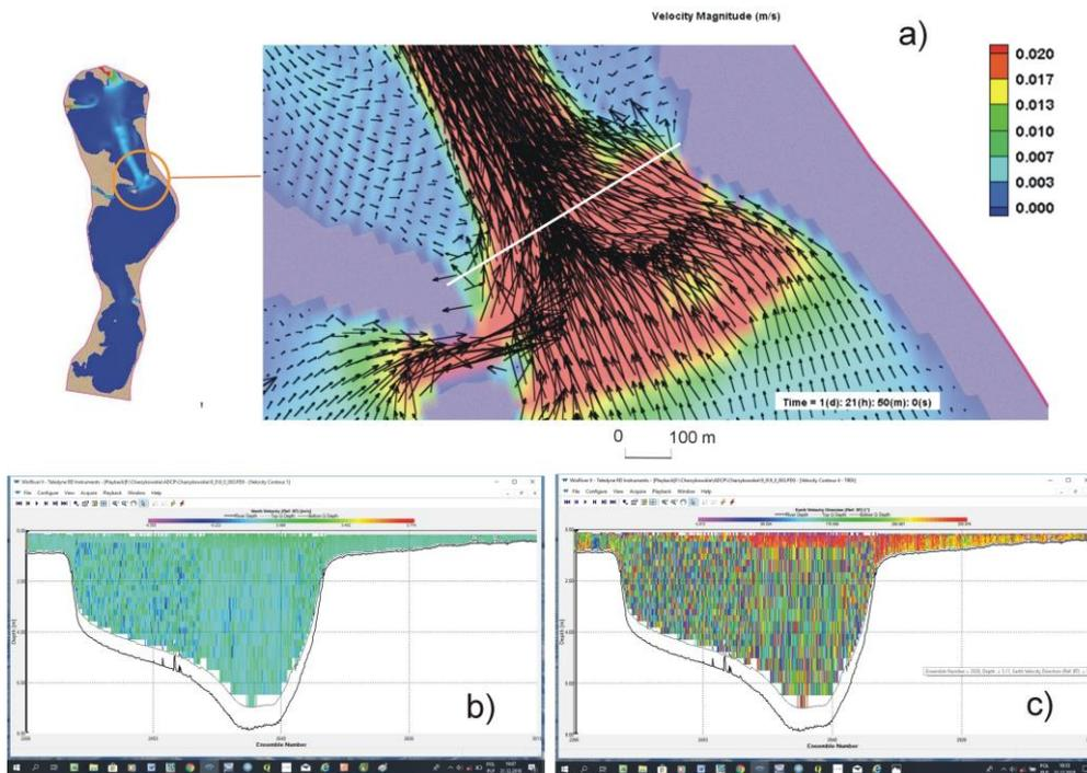
**Fig. 1.** Selected *ADCP* profile No. 9003 at sill separating sub-basins Central and Northern-2 compared to: a) velocity field calculated by *CCHE2D* model, b) velocity magnitude by *ADCP* measurement in geographic N direction, c) geographic flow directions by *ADCP* measurement
