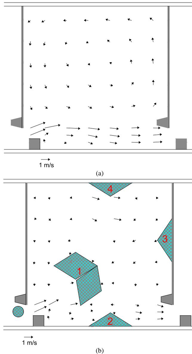
**Fig. 1** Velocity field in horizontal plane at  $z/d=0.32$ : (a) without brushes, and (b) with brushes in a vertical slot fish pass
