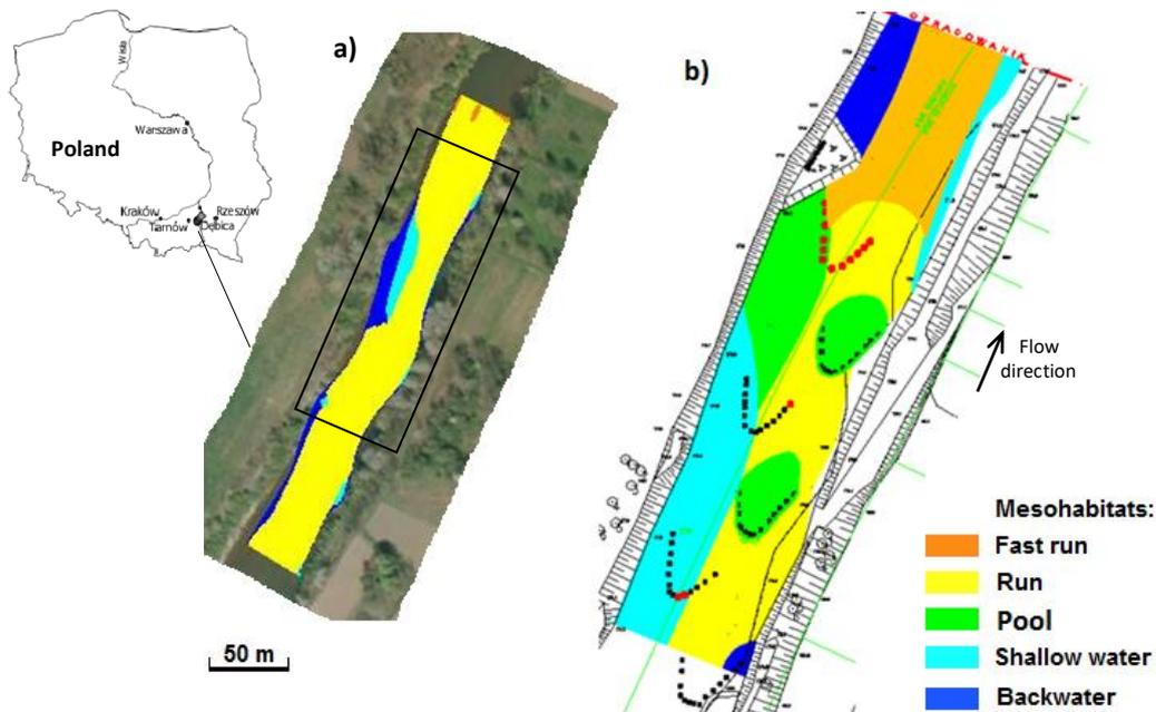
Fig. 1 Mesohabitats structure in the section number 10 of the Wisłoka river; a) before restoration, the 2D model for discharge  $Q=7.95 \text{ m}^3\text{s}^{-1}$ , b) after restoration, discharge  $Q=13.6 \text{ m}^3\text{s}^{-1}$ ; black and red symbols - restoration design
