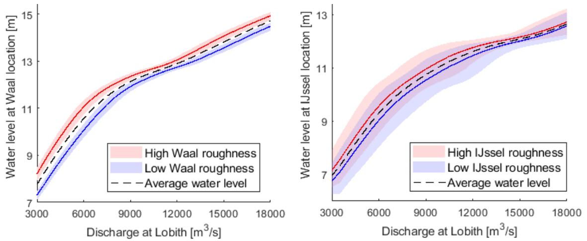
**Fig. 1.** Modelled water levels under the roughness scenarios for a Waal and an IJssel location. The left figure shows that the effect of the Waal roughness has a large influence on the water levels in the Waal, while there is only a narrow bandwidth around the modelled water levels. The right figure shows that the IJssel roughness has a minor influence on the local water levels, while a varying roughness in the other branches cause large variations in the modelled IJssel water levels.
