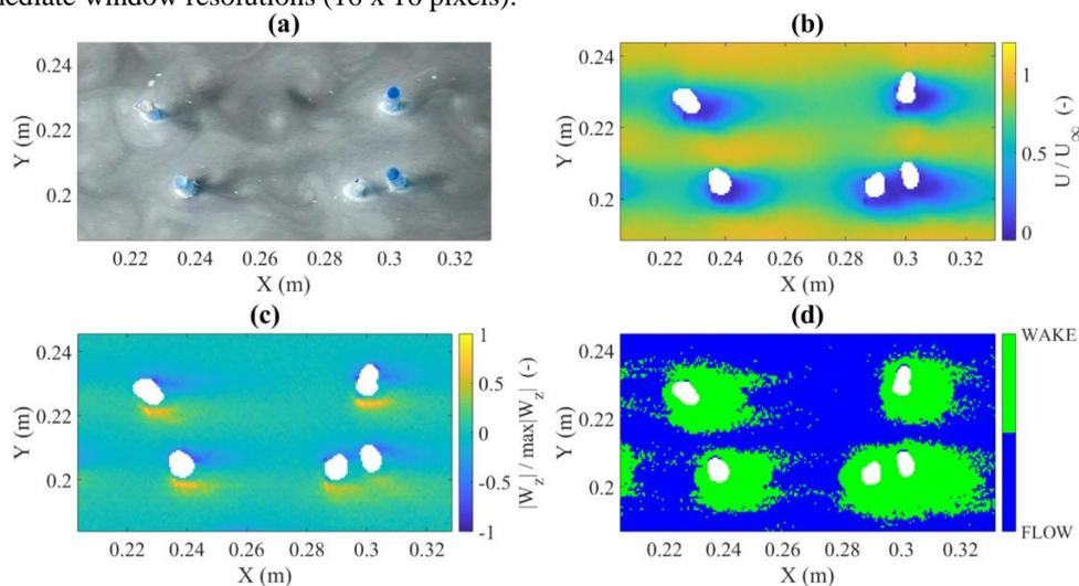
**Fig. 1.** Defined criteria to determine the wake area in flow through emergent vegetation. (a) Sample experimental section. (b) Time-averaged longitudinal velocity, as a fraction of the free stream velocity. (c) Time-averaged vorticity, as a fraction of the maximum absolute value of vorticity. (d) Wake area, shown in green for velocity fractions below 50% and vorticity fractions above 10%, respectively.
