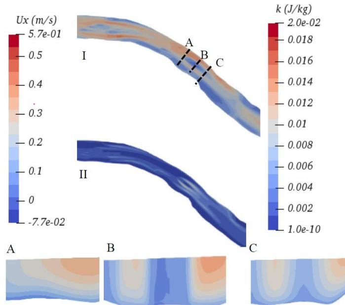
**Fig. 2.** Spatial distribution of streamwise velocity (I) and TKE (II) including cross-sections showing velocity changes within an individual patch.
