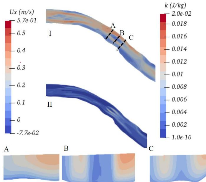
**Fig. 2.** Spatial distribution of streamwise velocity (I) and TKE (II) including cross-sections showing velocity changes within an individual patch.
