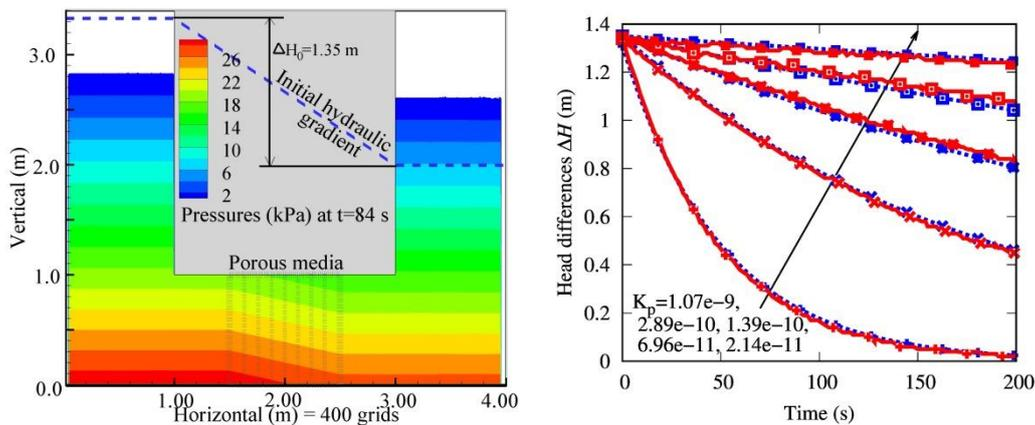
**Fig. 1.** Temporal hydrostatic pressure evaluation by the FS-IB-LBM at  $t = 84$  s in case of  $K_p = 1.07 \times 10^{-9} \text{ m}^2$  representing the U-tube porous media flow problem (left) and comparison between the analytically and numerically defined head differences in cases (right).
